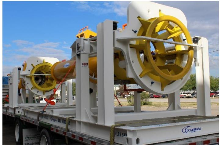
Figure 1 Static Mixer Module (SMM) installed within OceanWorks recently delivered Handling Aid ready for road transport.
